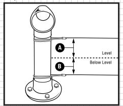
Measure the exact vertical height on the tallest side of panel. Record your measurements on the SOLARSCRIM ORDER FORM as indicated. Round down the measurements to the nearest quarter of an inch for any fractions. For example: 4' 3½".
