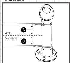
Any vertical coordinates that are below the level line must be noted on your SOLARSCRIM ORDER FORM. For example, if the vertical dimension is a total of 36" of which 5" are below the level line, Your measurements should read;
