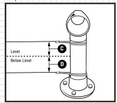
Measure the exact vertical height on the shortest side of panel. Record your measurements on the SOLARSCRIM ORDER FORM as indicated. Round down the measurements to the nearest quarter of an inch for any fractions. For example: 2' 21/4".
