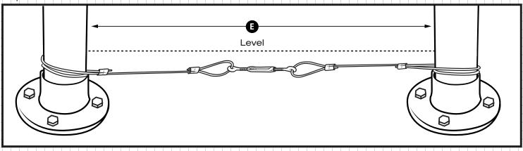
Measure exactly end to end at the level position along the bottom cable. Record your measurements on the SOLARSCRIM ORDER FORM as coordinate point E using whole numbers for feet and inches. Round down the measurement to the nearest quarter of an inch for any fractions. For example: 10' 234".
